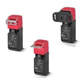
The STNK series is a key operated safety interlock switch designed to fit at the leading edge of sliding, hinged or lift-off guards. With its dual entry slots and rotatable head, the versatile STNK series can offer up to eight different actuator entry options.
