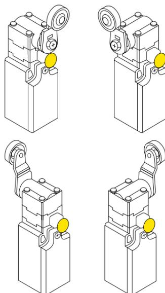
In all switches, it is possible to rotate the head in 90° steps.
