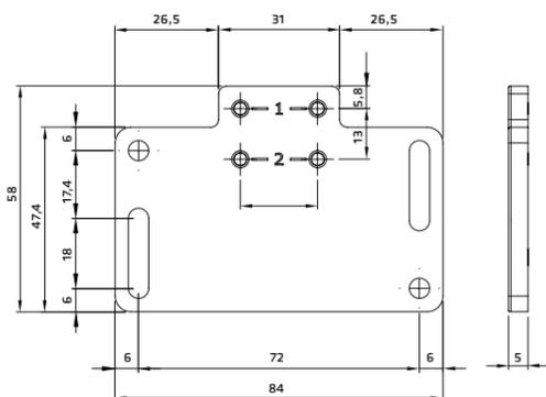
Fixing plate equipped with large slots for adjusting the operating point developed for backwards compatibility with old products. Each plate has a double pair of fixing holes.
